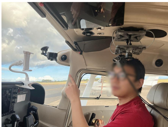
FIGURE 11. Setting up the shock-absorbing fixture for the cockpit camera in a Cessna 172S. © Mahdi Al-Husseini 2023
