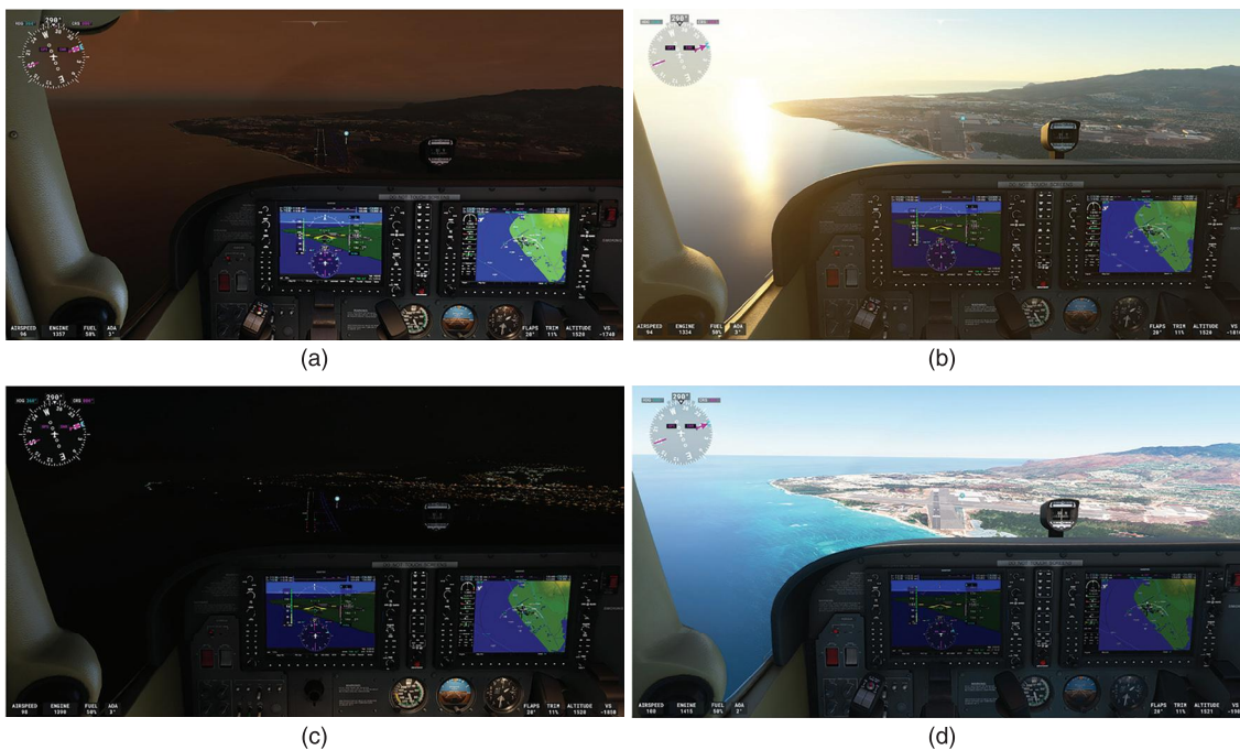
FIGURE 4. Digital flight simulation data recordings and video capture for a Cessna 172 G1000 executing an approach into Kalaeloa airport (PHJR) in varying environmental conditions: (a) sunset with an overcast cloud layer, (b) sunrise with clear skies, glare present, (c) nighttime with scattered clouds, and (d) high noon with clear skies.
